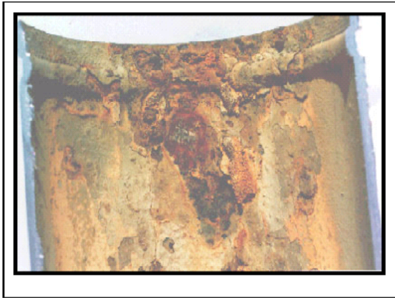
Corrosion at roll groove in a wet pipe system
