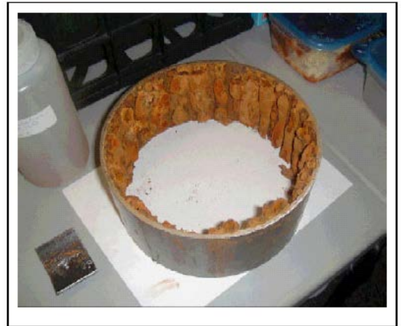
Heavy tubercle formation in a 8 in. sprinkler pipe
