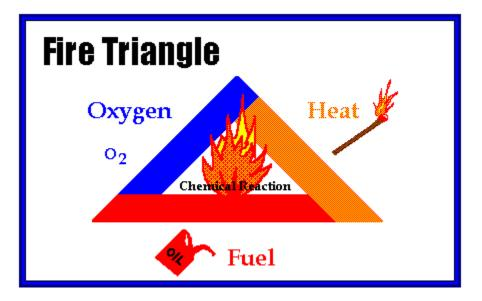
Oxygen, heat, and fuel are frequently referred to as the "fire triangle." Add in the fourth element, the chemical reaction, and you actually have a fire "tetrahedron." The important thing to remember is: take any of these four things away, and you will not have a fire or the fire will be extinguished.
